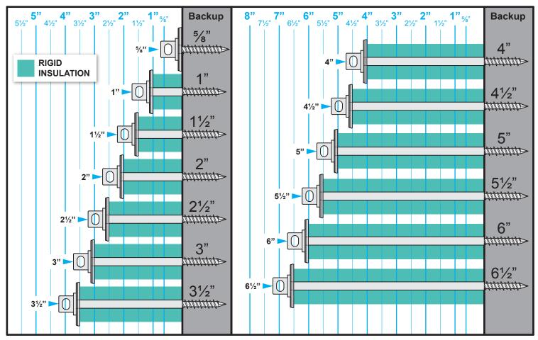
Concrete Seal Tie™ is an innovative single screw veneer tie suitable for use with concrete, CMU, wood stud, or brick backup. (for wood stud refer to wood stud size and selection chart)
