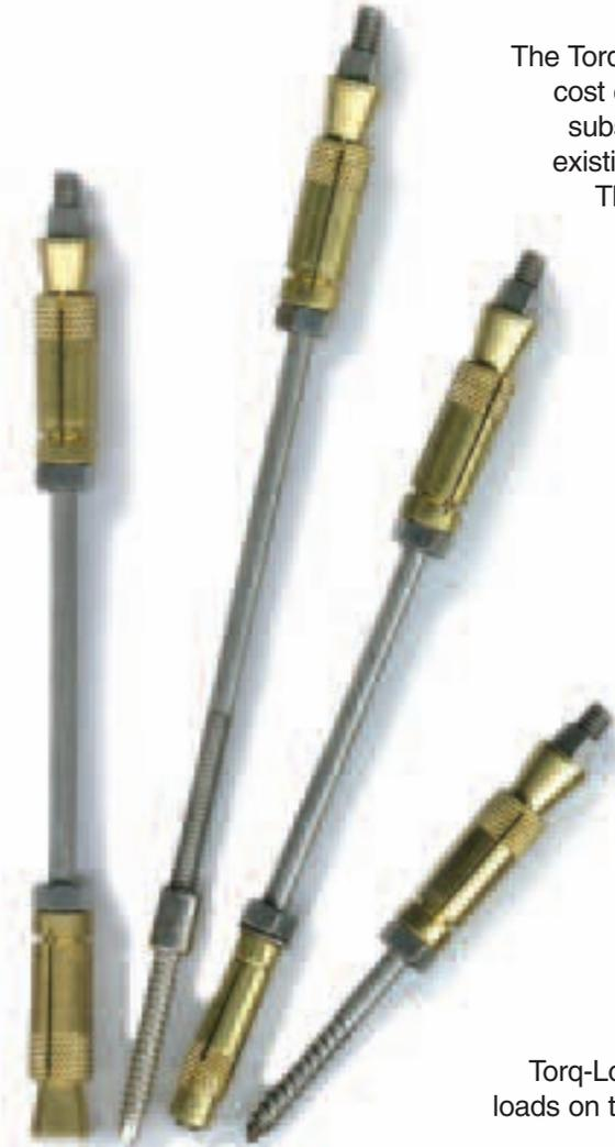
The Torq-Lok mechanical anchoring system is an easy to use and cost effective method to re-connect existing veneers to various substrates. The process eliminates the need to tear down an existing veneer by providing a corrosion resistant tie assembly. The components are manufactured of AISI Type 300 series austenitic stainless and ASTM Type 360 brass. The combination provides for long-term durability and structural stability for the design life of the structure.
