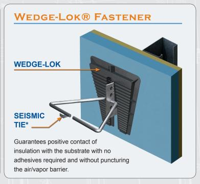
\*Seismic Flex-O-Lok Tie available for standard 407 or 407S Shear anchor allows for easy installation of continuous wire in seismic applications.
