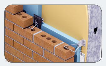
Recommended minimum spacing of one tie per 2.67 square feet of wall area, spaced not more than 32" horizontal, and 18" vertical in the U.S.; 24 in. horizontal (600 mm.) x 32 in. vertical (800 mm.) per CSA.
